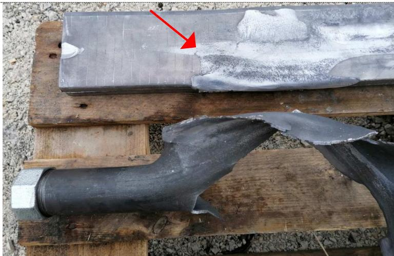
**Figure 3.** DDT results for rifle powders (UN0161; 1.4C)
