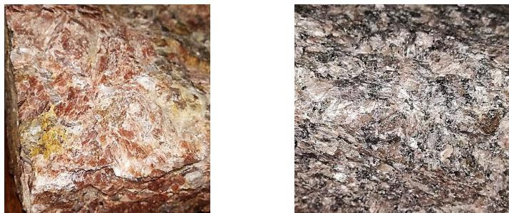
Figure 2 - Zverkivsky deposit granites extracted by the BWS method: a) - red granite, b) - gray layered granite
