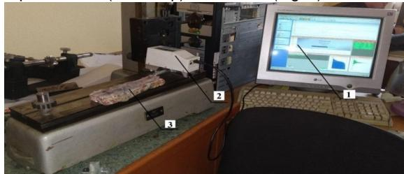
Figure 7 - Stand for measuring surface roughness: 1 - PC display; 2 - portable profilometer (workshop) RT-10 Plus; 3 - the test sample.
