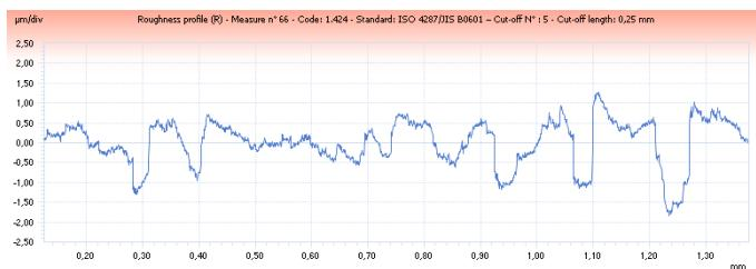
Figure 8 - Profile roughness curve (1 time - 315 mm / min) and its performance
