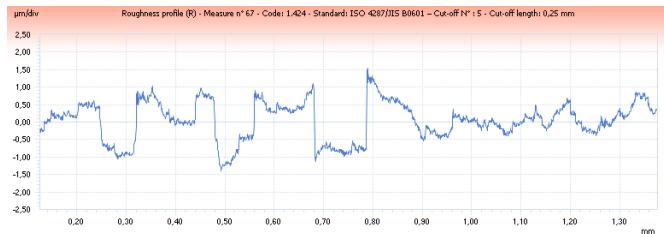
Figure 9 - Profile roughness curve (2 times 800 mm / min) and its performance.
