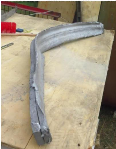
**Figure 2.** DDT lead anvil deformation results for shotshell powders (UN 0161 1.3C)
